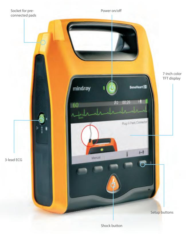
BeneHeart D1 has the high protection level (IP55) to against the dust and water.
