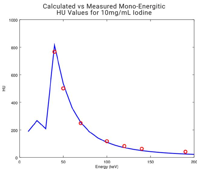
HU values of iodinated rod for mono-energetic reconstructions. Calculated values based on material compositions and NIST values (blue curve) vs HU values from mono-energetic reconstructions (red circles).
