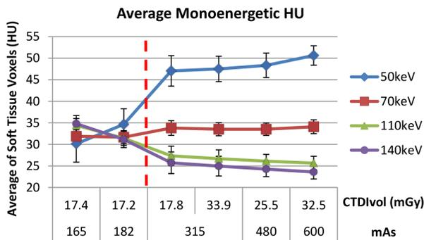
Average soft tissue monoenergetic HU for 50, 70, 110, and 140 keV reconstructions versus mAs, averaged over a 1 year period. Protocols left of the red dashed line were insufficient to provide reliable HU values.
